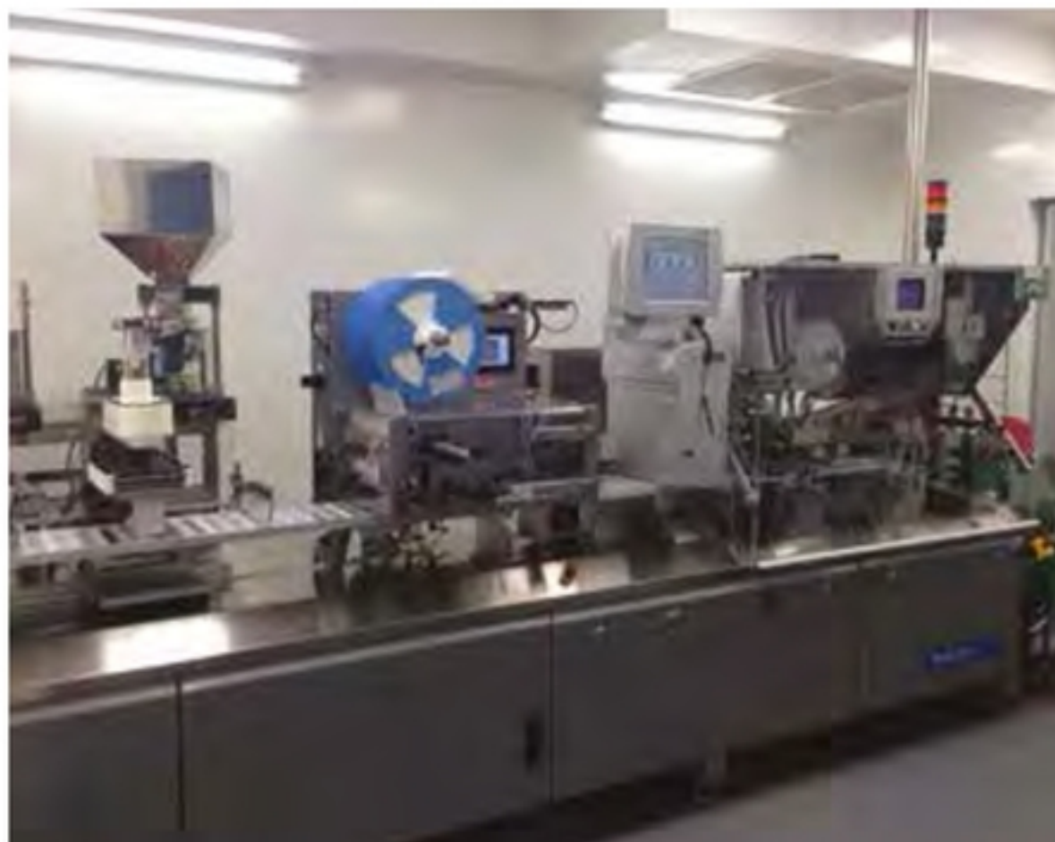
Romaco Noack 623 blister packing machine has provided flexibility for Almac Group
