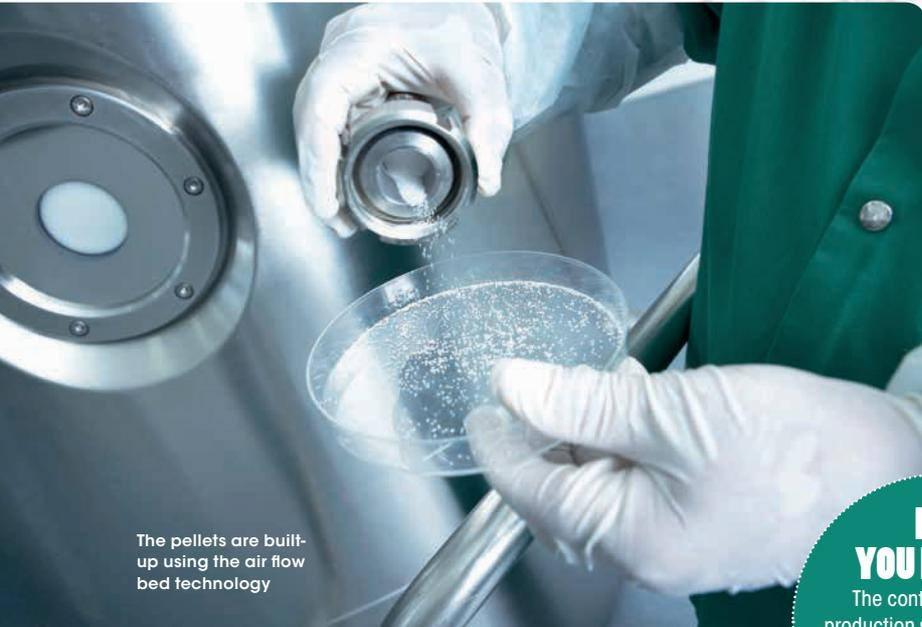
The pellets are built-up using the air flow bed technology
