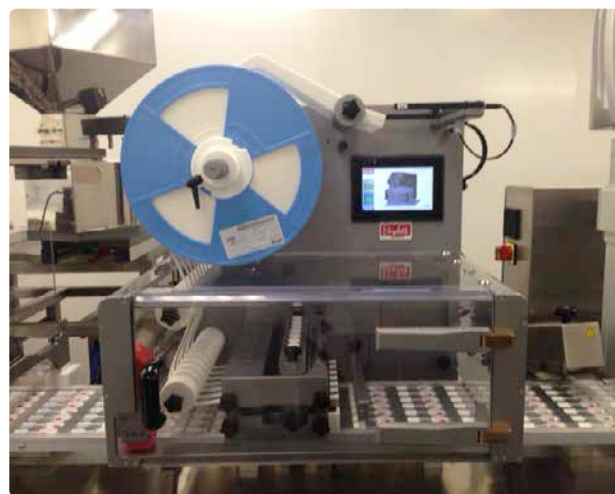
The Romaco Noack 623 blister machine installed at the Almac facility in Northern Ireland.
