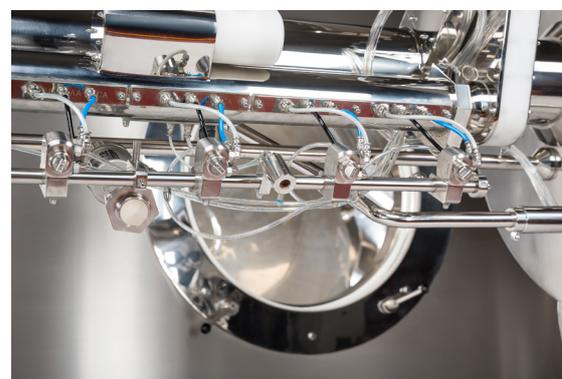
Automatic extendable spray arm with self-adjusting movable spray nozzles allows for variable batch sizes from 10% to 100%.
