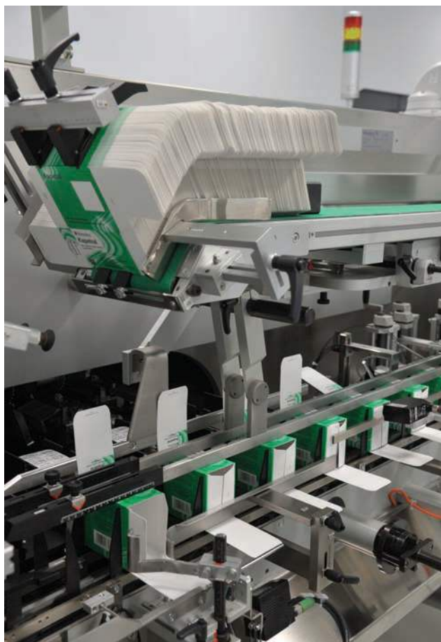
The blisters are packed in cartons on a Romaco Promatic carter
