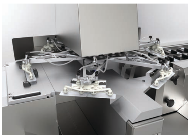
Stack transfer unit of the Romaco Noack Unity 600
