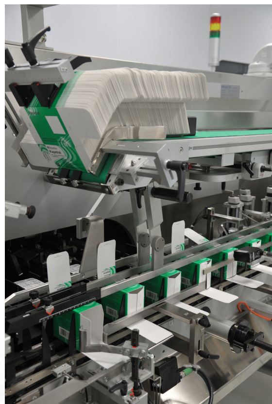
The blisters are packed in cartons on a Romaco Promatic cartoner (Image: Romaco)
