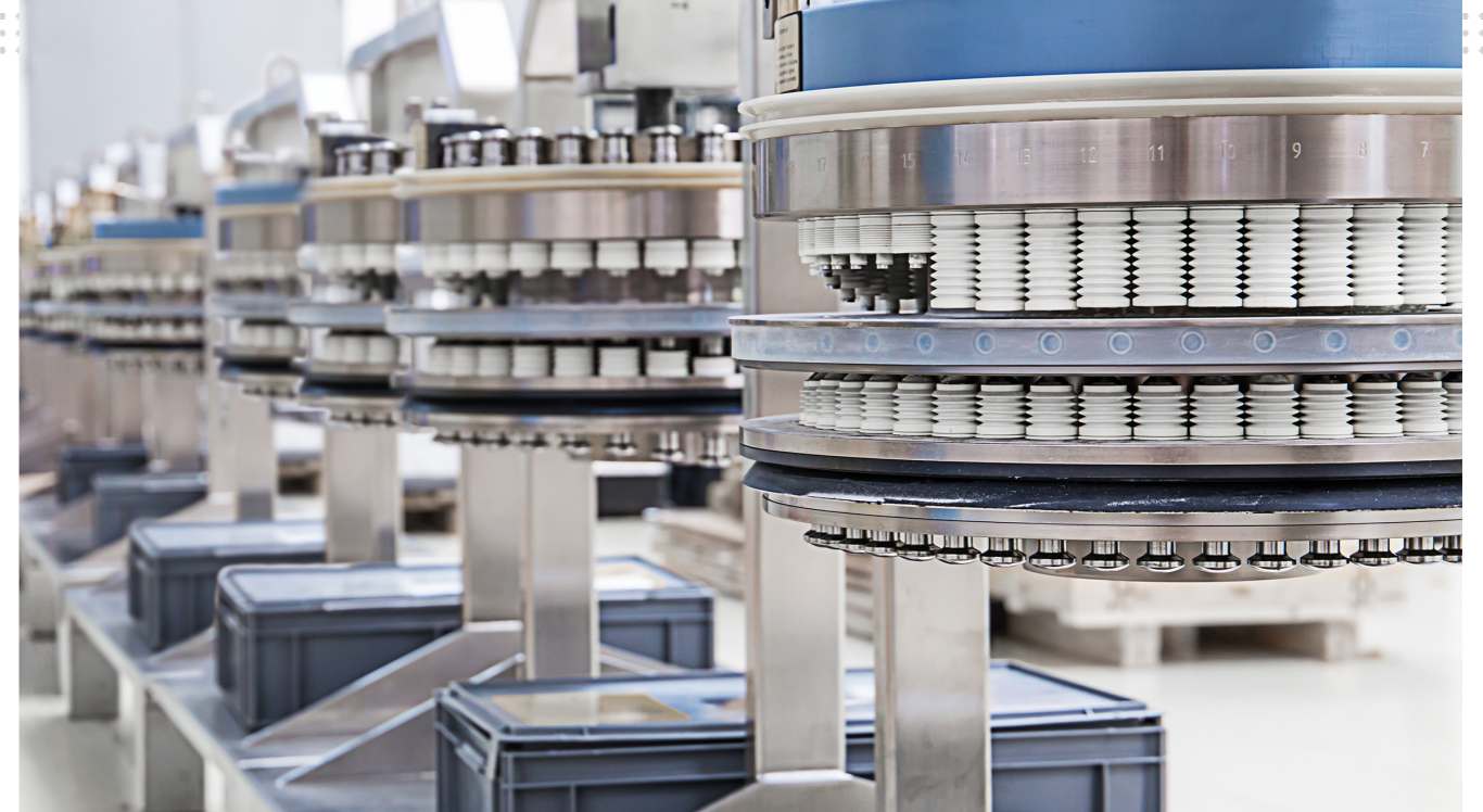
The use of identical die tables helps optimise the OEE and TCO of the tablet press (Image: Romaco)
