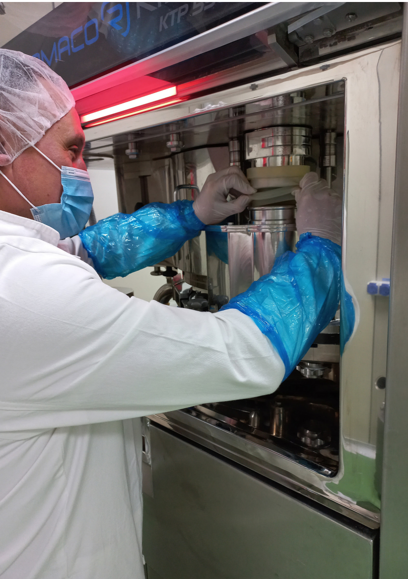
A single machine operator requires just 10 to 15 minutes to install the interchangeable parts and the die table (Image: Hemofarm)
