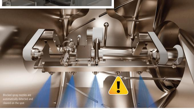
More efficient drying and the ability to make adjustments without interrupting the coating process reduce production times by hours The batch volume and the tablet bed inclination are measured continuously using sonar technology
