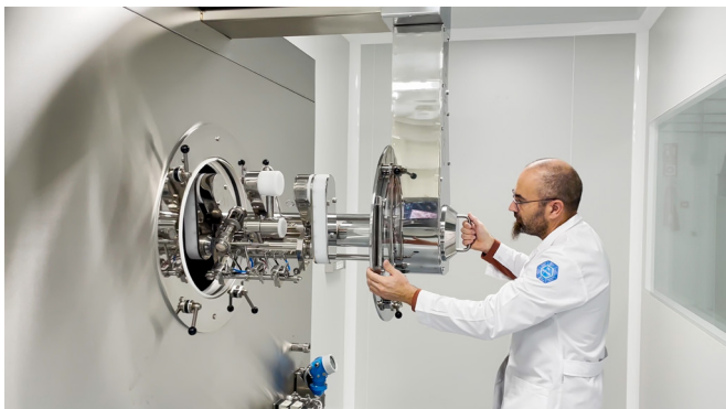
The TPR Optima tablet coater from Romaco Tecpharm creates a reproducible coating process
