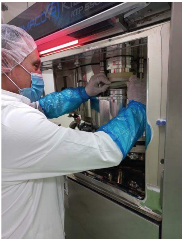
A single machine operator requires just 10 to 15 minutes to install the interchangeable parts and the die table
