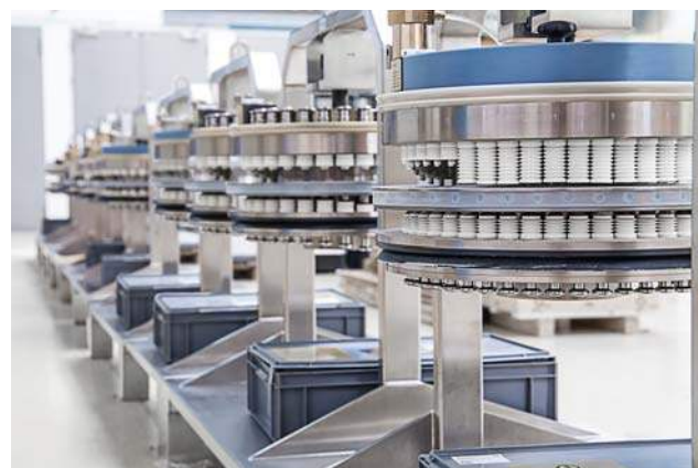
The use of identical die tables helps optimise a tablet press's OEE and TCO
