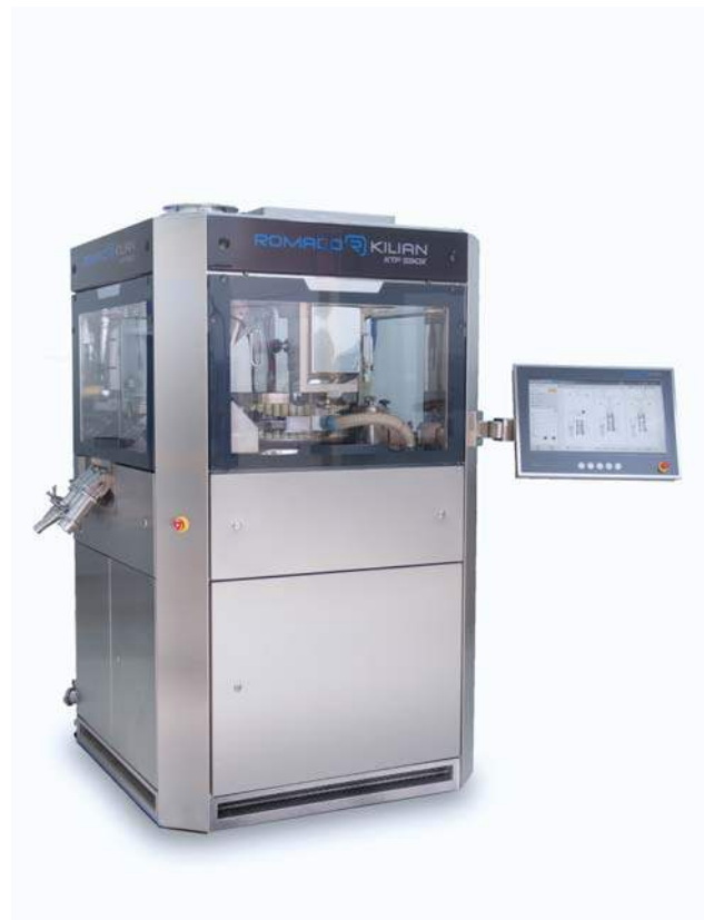
The KTP 590X high-speed press is in use at Hemofarm 24/7 and is completely retooled and cleaned once or twice a week
