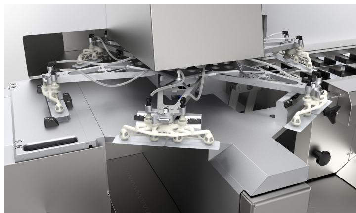
Blister transfer with the Romaco Noack Unity 600's indexing wheel
