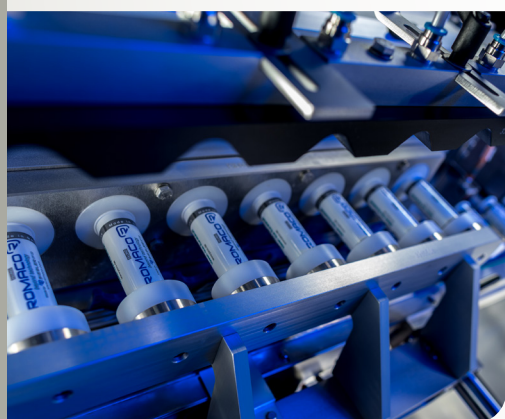
Effervescent tablets are filled carefully according to the rotation principle using the Romaco Siebler STF 120 tube filling machine
