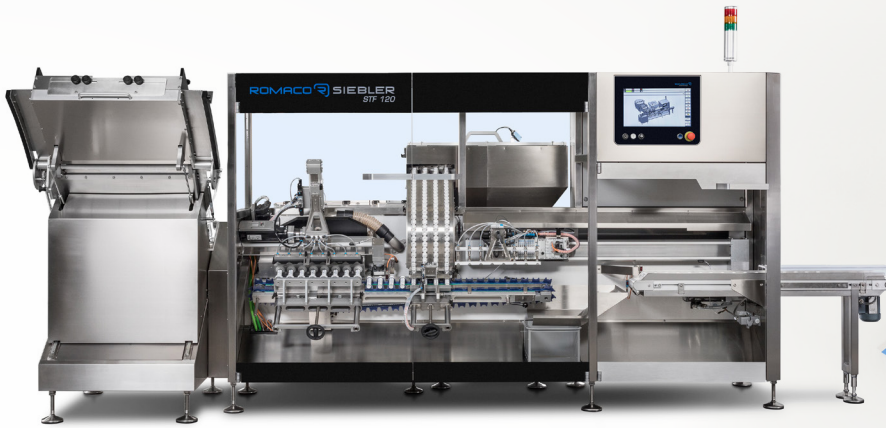
Under a development collaboration arrangement, Hermes Pharma was involved in the design of Romaco Siebler's STF 120 tube filling machine
