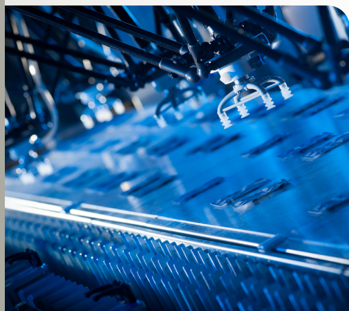
With up to 900 picks per minute, the Siebler FlexTrans is said to be the world's fastest transfer unit for strip packaging
