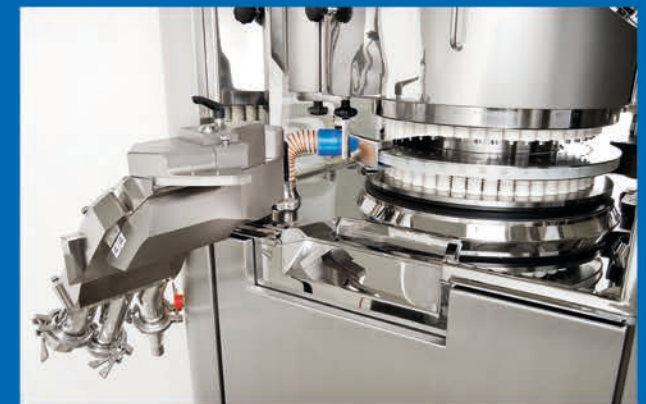
Dust-tight tablet chute mounted on swivel arm
