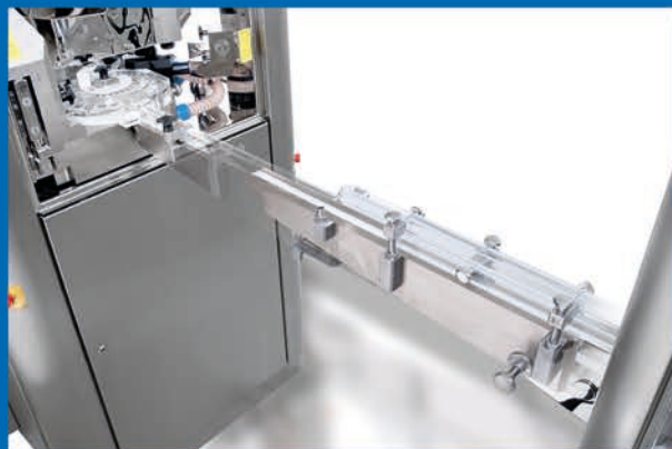
Conveyor belt for core distributor with sliding mechanism for better access
