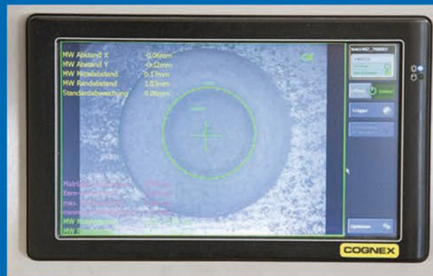
Camera and HMI with separate monitor for core position details
