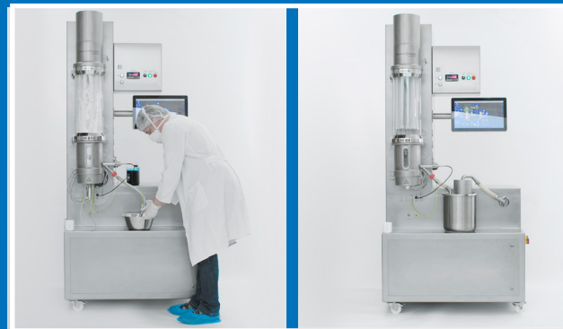
Pneumatic filling and pneumatic discharge
