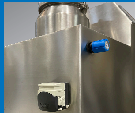
Automatic addition of binder solution with peristaltic dosage pump
