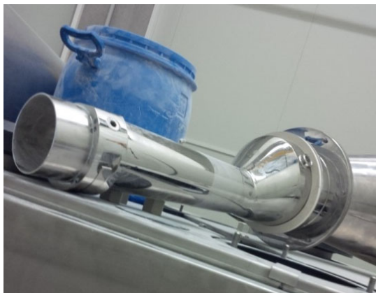
Conical filling tube for better product flow
