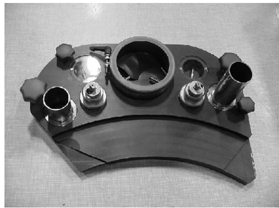
Fill shoe with chimneys for better de-aeration
